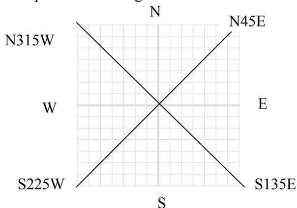
Set a point: The point measured from the transit at a given distance and bearing.
